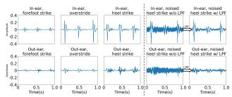
Fig. 2: In-ear (upper row) and Out-ear (lower row) signals of three running gaits and a noisy heel strike gait signal. speeds. However, heel strikes can exert additional strain on
