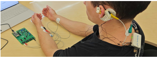
Fig. 2. Experimental Setup: MAX30001G evaluation board recording ground truth Lead I ECG at the wrists, and OpenEarable-based system recording heart sounds from the ear canal and ear-ECG signals
