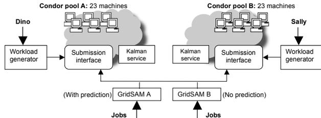
Figure 5. Test-bed Architecture.
