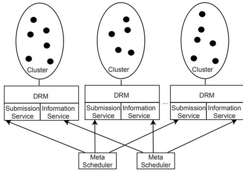
**Figure 4. Architecture of Grid environment**
