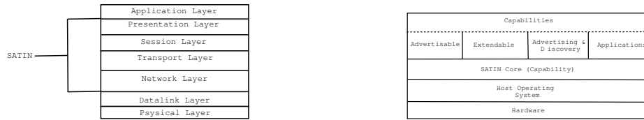
Fig. 2. (a) Our architecture in the context of the ISO/OSI networking model. SATIN capabilities represent the network, transport, session and presentation layers. (b) A high level view of SATIN. It is composed of modules, or capabilities, registered with a core.
