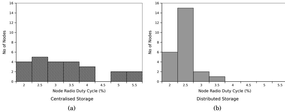
Fig. 10. Results from the network test: (a) Distribution of node duty cycles for the centralized storage approach. (b) Distribution of nodes duty cycles for the distributed storage approach.
