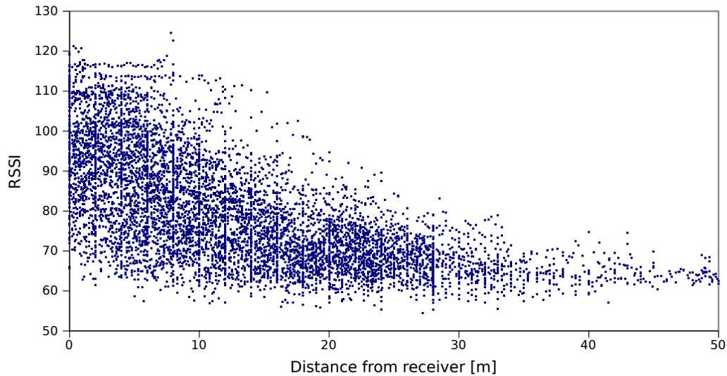
Fig. 5. Variation in RSSI of RFID detection nodes with distance.
