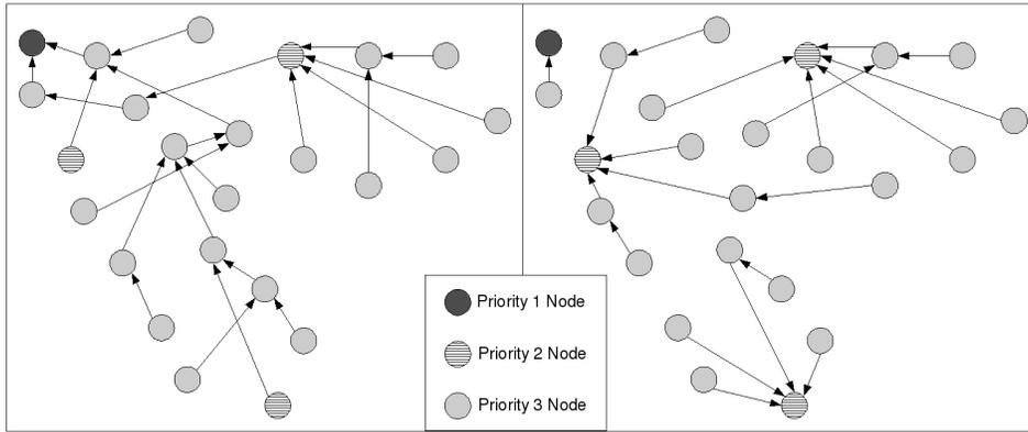
Fig. 9. Example routing trees as found in our deployment: (left) Routing tree for priority 1 data, (right) Routing trees for priority 2 data.
