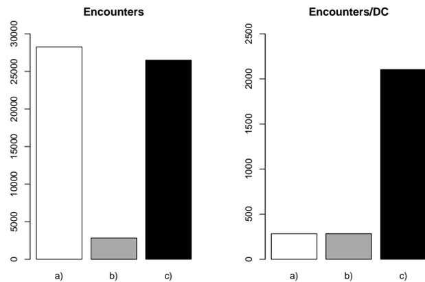
Fig. 13. Deployment results with new hardware. Comparison of detected encounters and encounters per effective duty cycle for a) always-on b) fixed c) adaptive algorithms.
