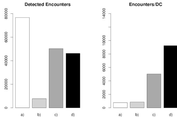
Fig. 7. Simulation results. Comparison of detected encounters and encounters per effective duty cycle for a) always-on b) fixed c) short-term adaptation d) short-term and long-term adaptation.
