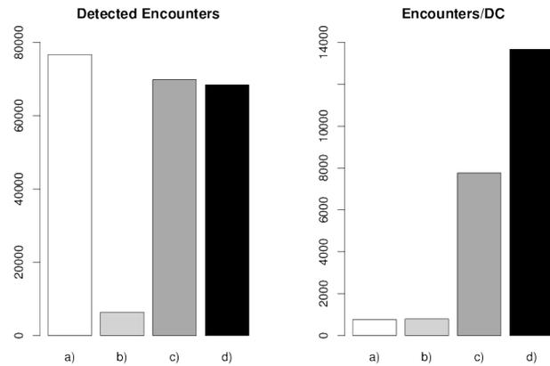
Fig. 12. Simulation results. Comparison of detected encounters and encounters per effective duty cycle for a) always-on b) fixed c) short-term adaptation d) short-term and long-term adaptation.
