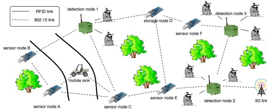
Fig. 2. Heterogeneous network consisting of badgers (equipped with RFID collars), detection nodes (fixed RFID receivers), environmental sensor nodes, zoologists (mobile sinks) and a fixed gateway.
